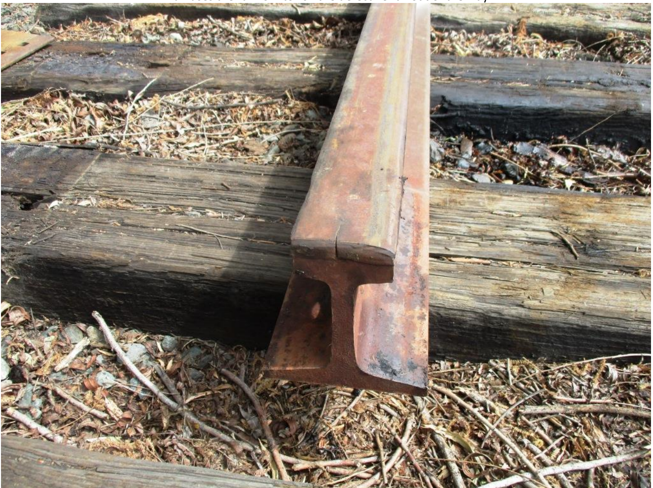
The culprit – a vertical split rail-head
