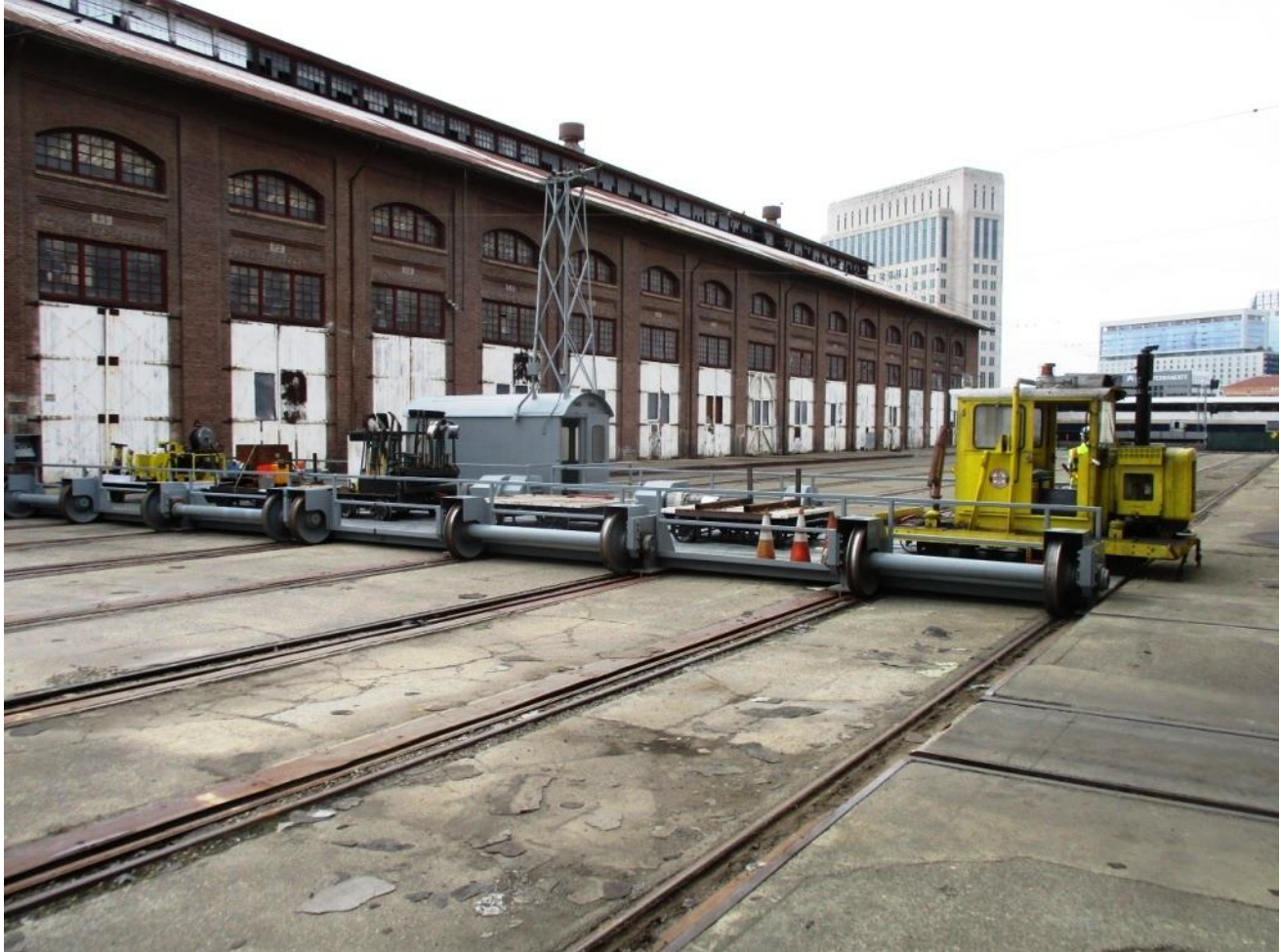
A transfer-table full: the Kalamazoo grabs all the needed equipment MOW equipment out of the Shops
