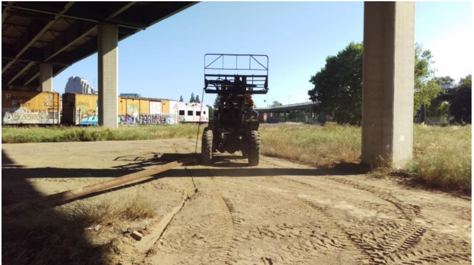
Big Green drags a stick of 110-pound rail out of the spare rail pile
